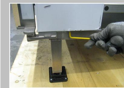
Use a size 4 Allen key to undo the screw at the bottom of the slide-panel cover.
